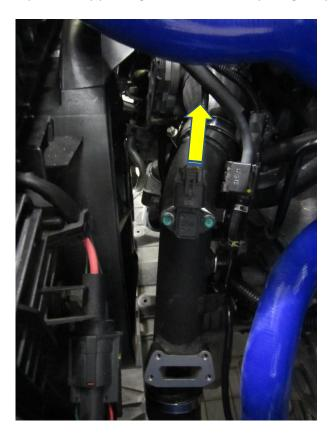
7. Using long nose plyers loosen the sprung hose clamps securing the small vacuum hose from the solenoid to the boost pipe and remove the pipe completely. Using a 10mm socket and ratchet remove the M6 fastener holding the solenoid to the OE boost pipe.
