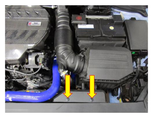
3. Using a spring clamp removal tool or long nose pliers compress the spring clip so that you can slide it down the hose and remove the inlet pipe.
