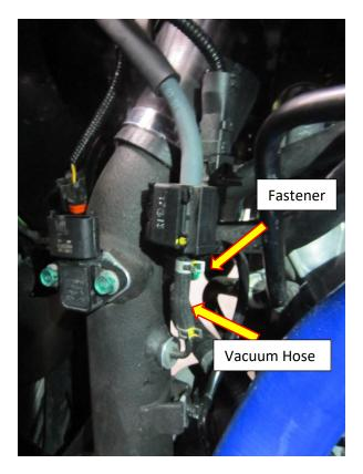
8. Move the solenoid and map sensor loom out of the way to make the removal of the boost pipe easier.
