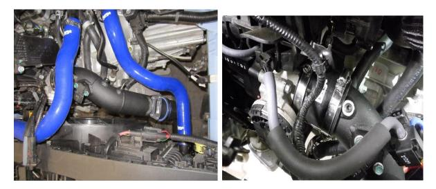
13. Mount the solenoid to the FMBP7 hard pipe using the m6 fastener removed earlier. Use the vacuum hose supplied with the kit to replace the original hose as this will be too short to reuse. This needs to be used for the diverter valve vac hose also, Cut the vacuum hose to the required length with the use of side cutters then use the provided small cable ties to secure the vacuum lines in place.
