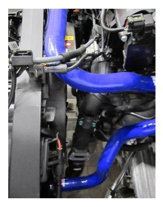
9. Using an 8mm socket and ratchet release both hose clamps attaching the boost pipe to the vehicle, there is one which holds the rubber joiner hose to the throttle body and one which holds the 90 degrees joiner hose to the intercooler. Some clamps may have a cover over the worm drive, this can be removed with plyers.
