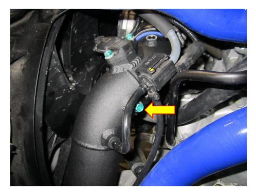
14. Re-fit the diverter valve and connect the vacuum hose, use the large cable tie to secure this vacuum hose to the lower radiator hose. Do not over tighten this as it can pinch the vacuum line.Using a 7mm sockt and ratchet tighten up all the hose clamps.
