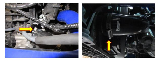
**10**. With the boost pipe out of the vehicle, use a 10mm socket and ratchet to remove the X 2 M6 fasteners attaching the map sensor to the boost pipe.
